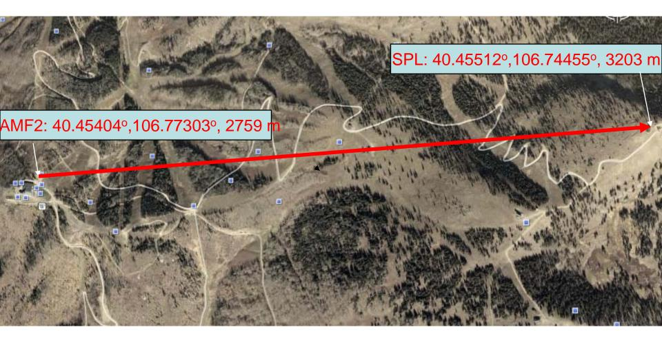
AMF2 - SPL distance: 2.4 km AMF2-SPL azimuth: 87.2°, AMF2-SPL elevation: 10.4°
