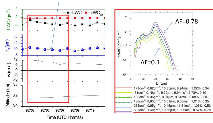
CAIPEEX 2009: LWC values measured at different heights in developing cumulus clouds observed : a) in premonsoon clouds developing in extremely polluted and dry atmosphere (June 16); b) transition period (June 21-) and c) monsoon clouds developing in moist and less polluted air (June -22, August 23, 24, 25).
