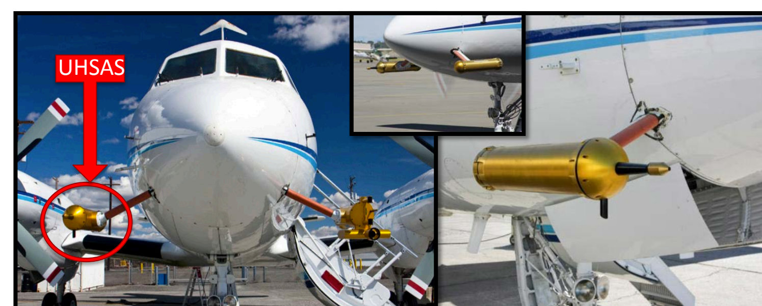
Figure 3. Tomlinson UHSAS deployed on G-1 Aircraft during CARES FC.
