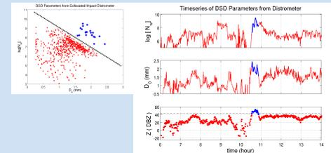
Partitioning agrees well with collocated surface-based impact disdrometer data to reveal multiparameter bulk drop size distribution (Bringi et al 2009) linked to the assigned radar-based regimes.
