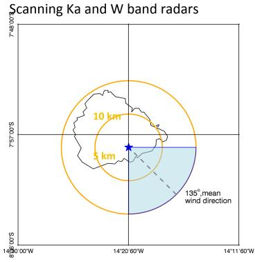
Radar will perform RHI scans over a 90 degree sector centred on the mean wind direction (blue shading). Co-ordinated flying in range of the radar.
