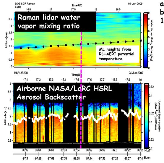
ML heights from RL+AERI potential temp. profiles and airborne HSRL aerosol backscatter measurements within 10 km and 10 min of SGP
