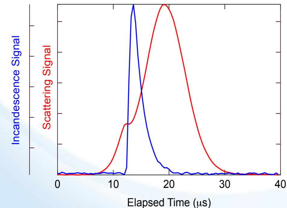
Pronounced asymmetry in the scattering amplitudes is attributed to rBC located near or at the surface of the 'host' material.
