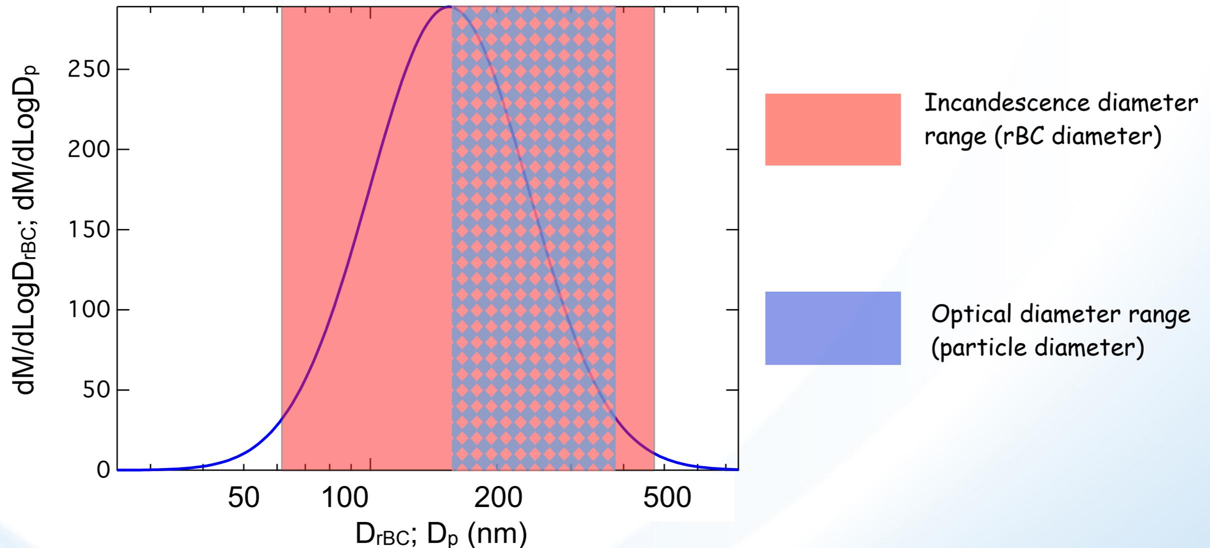
'Useful' diameter range for SP2-based BC mixing state analysis: ~160 - 375 nm
