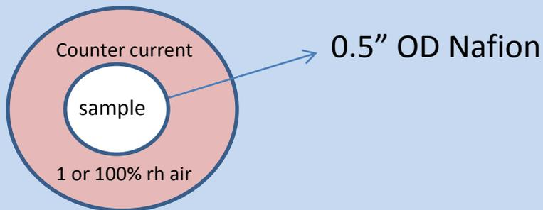
Needs source of 5-20 l/min of dried air ( $\sim 1\%rh$ ) and 5-20l/min humid air ( $\sim 100\%rh$ ).
