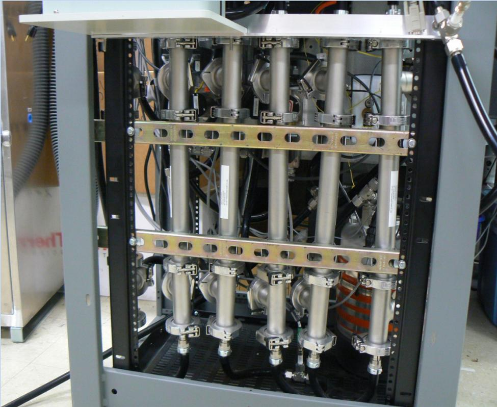
The aerosol humidifier part of the  $f(rh)$  consists of six Nafion permeation tubes, the first three are for preconditioning. The last three are the sample tubes. The aerosol sample is separated from the drying/humidify gas stream by the Nafion membrane.
