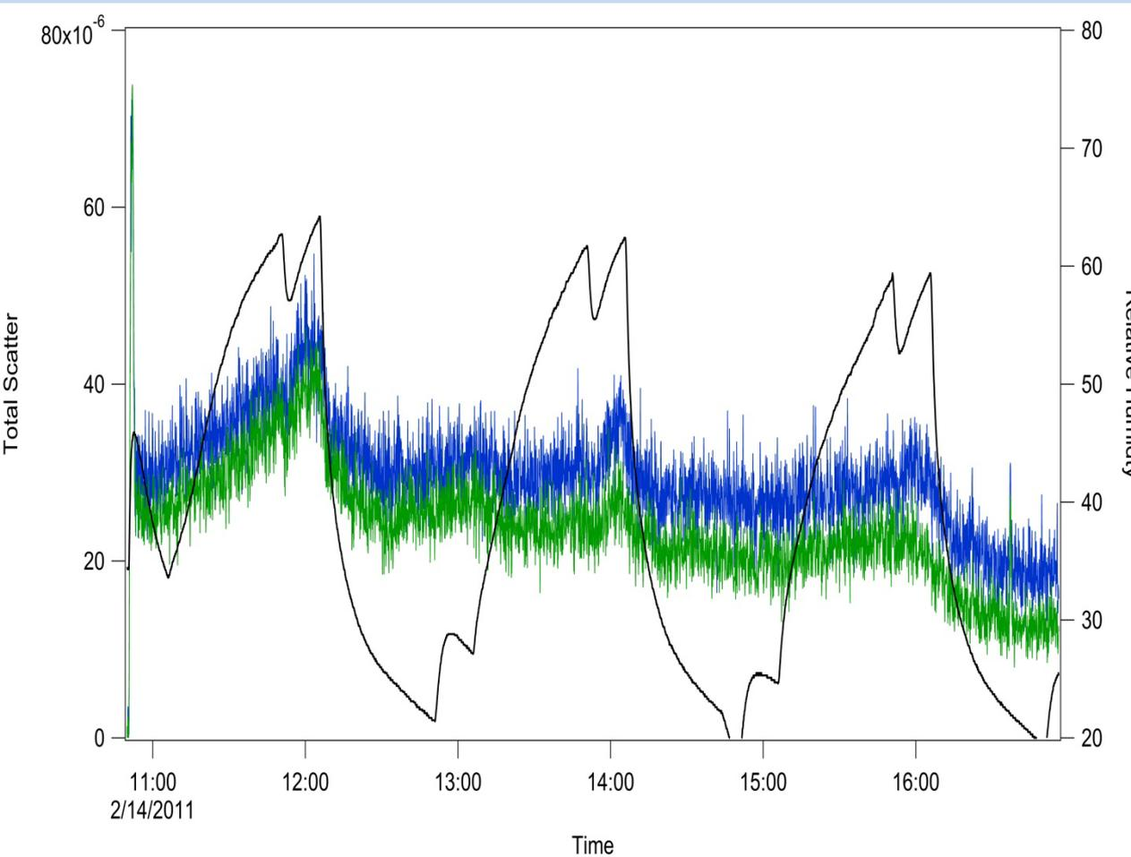
Note the maximum in the scattering every two hours corresponding to the maximum humidity in the deliquescence cycle
