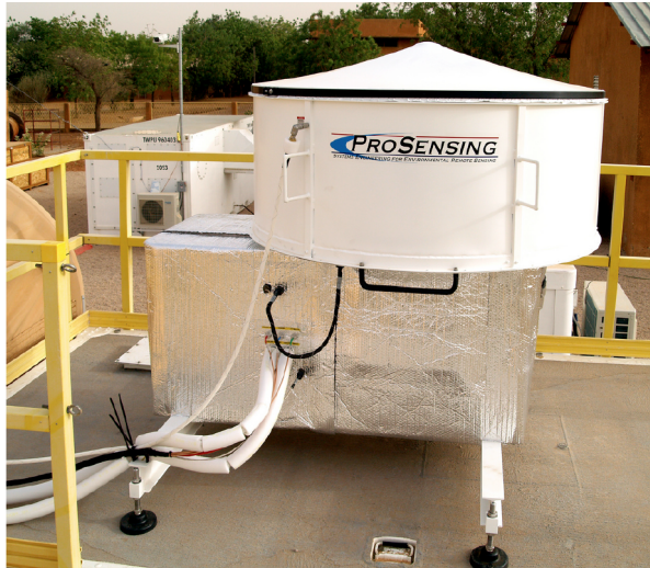
The W-band (95GHz) ARM Cloud Radar
