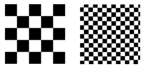
Optical thickness of cloudy and clear regions is 18 and 0.001; cloud fraction is 0.5; single scattering albedo is 1; and asymmetry parameter is 0.85.
