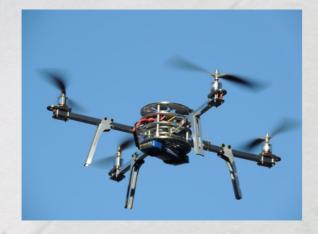
Overview: Small, lightweight quad- or hexa-copter with attached corner reflector and advanced navigation for precise height/position Advantages: Hovering capabilities, inexpensive Disadvantages: Operation in calm conditions
