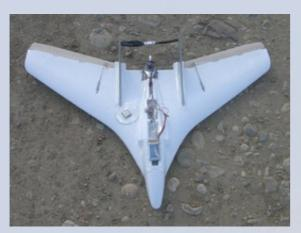
Overview: Small, lightweight (~700 g), inexpensive (~\$1000) UAS with basic meteorological instrumentation on board Advantages: Lightweight, cheap, relatively easy to operate, maneuverable Disadvantages: Small payload, limited endurance
