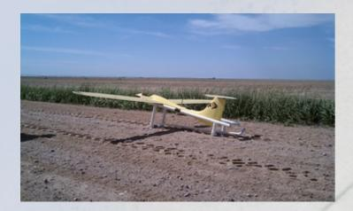
Overview: 10.5 ft. wingspan, I hour endurance, 75 kt. cruise speed, 15 lb. maximum takeoff weight Advantages: Larger payload capabilities, longer endurance Disadvantages: More expensive, front-mounted propeller Payload Demonstrations: cloud particle imager, broadband radiometers, aerosol counters
