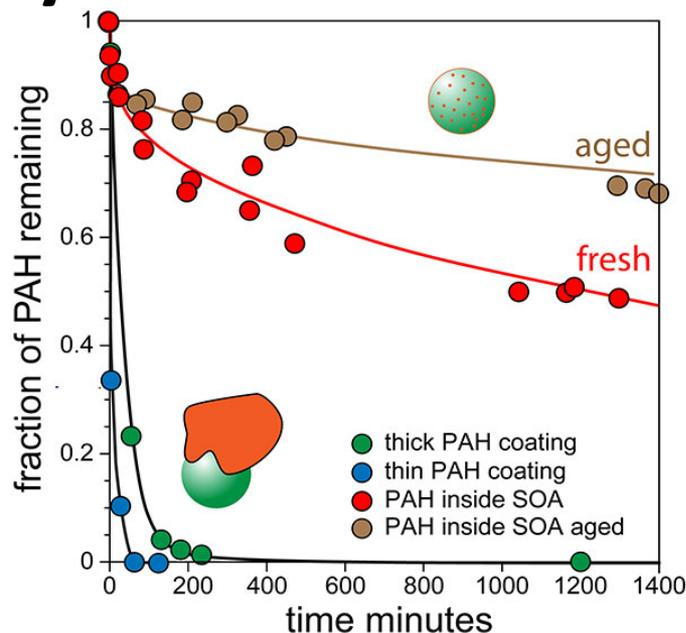
The evaporation rate of pyrene tracer-molecules trapped in SOA during its formation provides direct information about pyrene diffusivity in SOA and SOA viscosity
