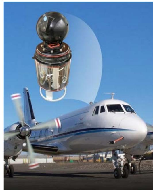
The 4STAR instrument (inset) is installed through the upper hull of the PNNL G-1 research aircraft, for in-flight sun-tracking and sky light-scanning.
