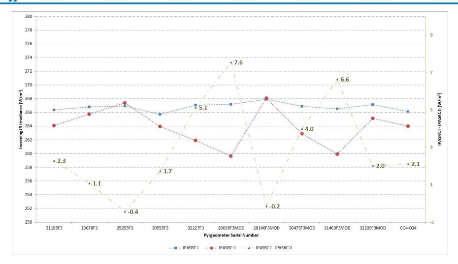
Calculated IR incoming irradiance measured by 11 pyrgeometers using their two sets of coefficients, derived during IPASRC I & IPASRC II
