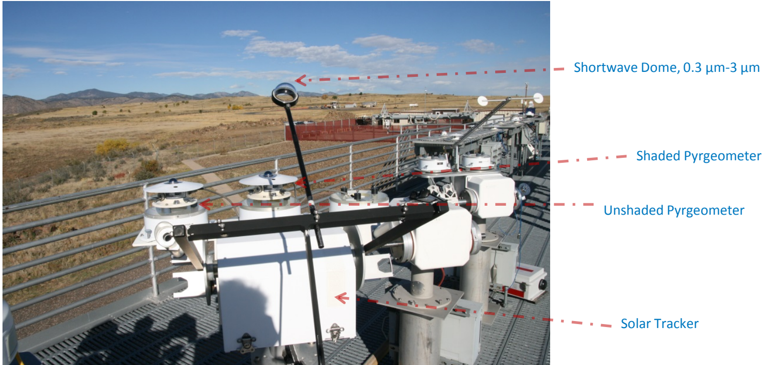
Figure 1. Unshaded and shaded pyrheliometers at NREL/SRRL
