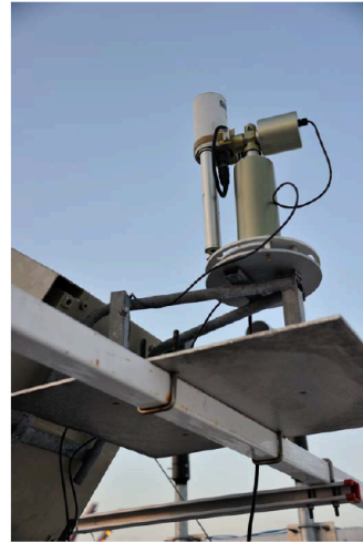
CIMEL Sunphotometer operated in cloud mode
