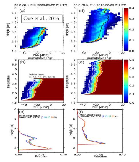
Contoured frequency by altitude diagram (CFAD) of radar reflectivity observed by the SACR (CR-SIM) with hydrometeor mixing ratios > 0.01 g/kg. Black line represents mean profile.
