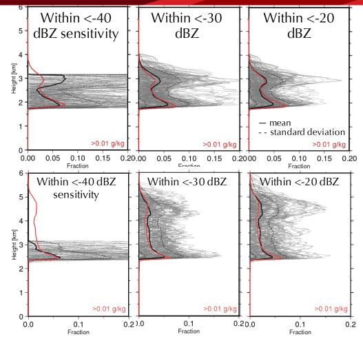
Cloud fractions from WRF mixing ratio greater than 0.01 g kg<sup>-1</sup> (red) and CWRHI scans (gray line), mean cloud fraction (black solid line), and standard deviation (dashed lines) for sensitivity regions of -40 dBZ, -30 dBZ, and -20 dBZ
