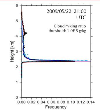
Red: WRF hydrometeor mixing ratio > 0.01 g/kg Blue: Lowest height of lidar (ceilometer) backscatter ( >  $10^{-4}$  sr<sup>1</sup>m<sup>-1</sup>) Black: Lowest height of Ka-band Zhh (- $50+20\log 10(R)$  dBZ is applied)
