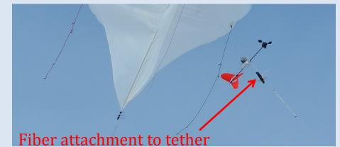
**Distributed Temperature Sensing (DTS) system** composed of **1.5 km** of fiber optic cable. The fiber optic cable serves as the thermometer, with a laser serving as the illumination source. Provides measurements of temperature every 2 meters every 30 seconds with temperature resolution of < 0.1°C. First flown on TBS at Oliktok on 4/18/16.
