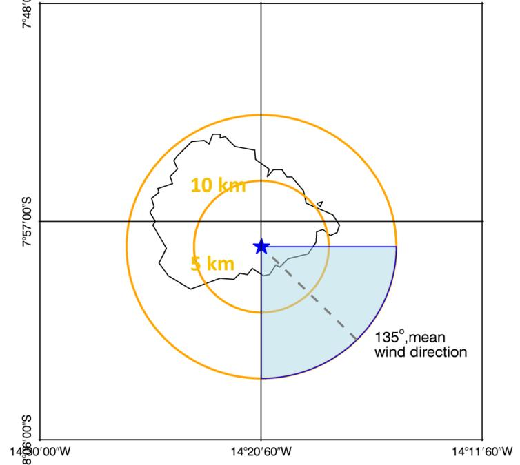
Radar will perform RHI scans over a 90 degree sector centred on the mean wind direction (blue shading).
