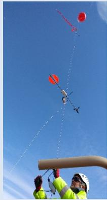
Tethersondes and radiosondes provide pressure, temperature, RH, and wind speeds. Turbulence pod in Oct '16.
