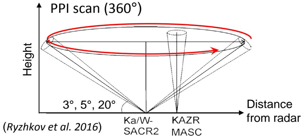
Azimuthal averages of polarimetric variables at each level from PPIs at three elevation angles (3°, 5°, 20°) every 30 min.
