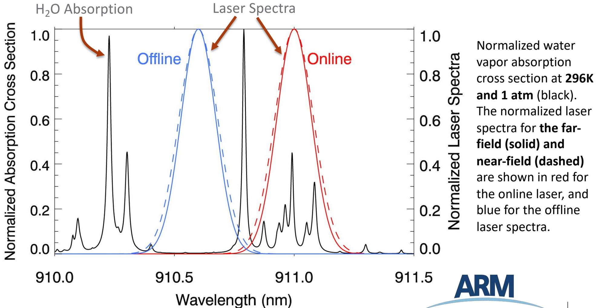
Normalized water vapor absorption cross section at **296K and 1 atm** (black). The normalized laser spectra for **the far-field (solid) and near-field (dashed)** are shown in red for the online laser, and blue for the offline laser spectra.
