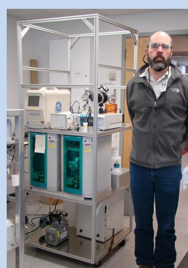
Shock mount PILS for MAOS. CO instrument to go at top (author for size reference)
