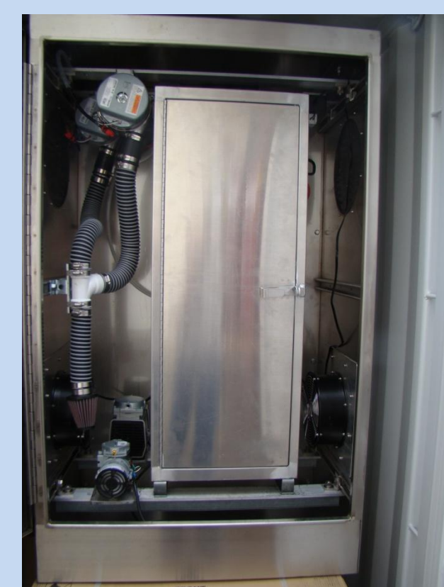
Add f(RH) and HTDMA driers to pump box
