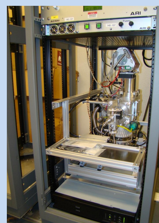
ACSM Unit #2 modified for rack mounting in TWP-D. Unit #1 operating at SGP, Unit #3 to go in MAOS
