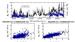
Babs coefficient for CARES campaign at T1 site. PASS-3 (10 min data) was not operating between 6/11 and 6/21. The scatter plots are for the 6/03 - 6/11 and 6/19 -6/28 operating periods. The overestimate of Babs by the PSAP corresponds with the coating enhancement. The PSAP operated with a 1 micron size cut off, the PASS-3 nominally transmits particles smaller than 2 microns.
