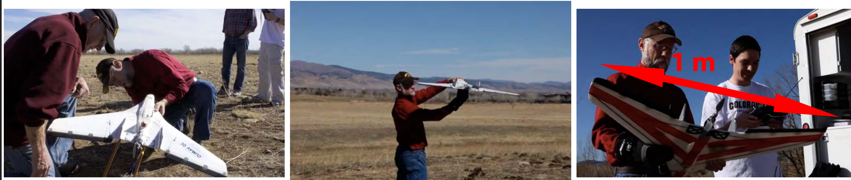
Photographs of the DataHawk in action in Colorado. The aircraft can be launched using a portable bungee launcher (left) or by hand (center). The right-hand image gives a good impression of the scale of the aircraft.
