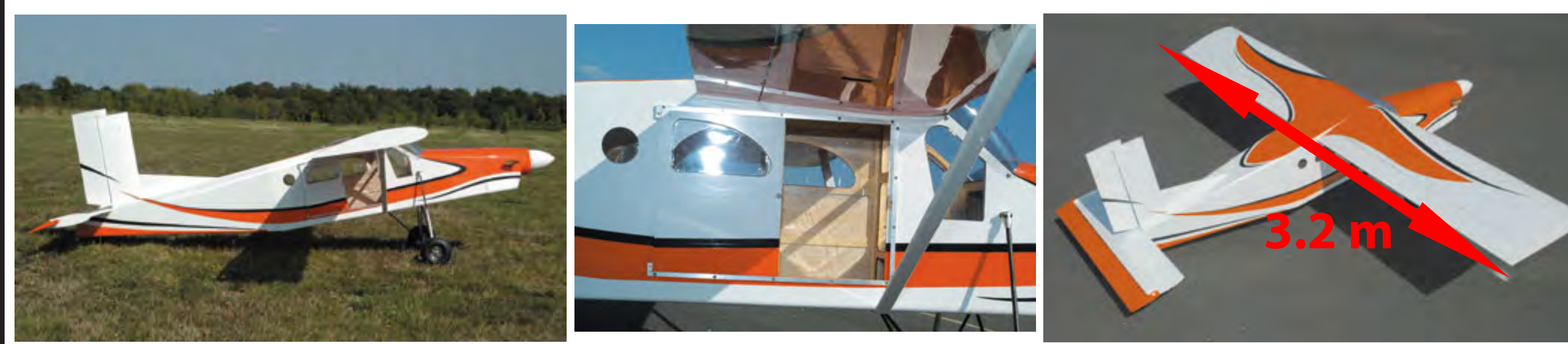
Photographs of the Pilatus aircraft. The left- and right-hand images provide insight into the scale and layout of the aircraft. The center image provides a better look at the space available for instruments inside the payload bay (dimensions of bay: 20"x9.5"x12").
