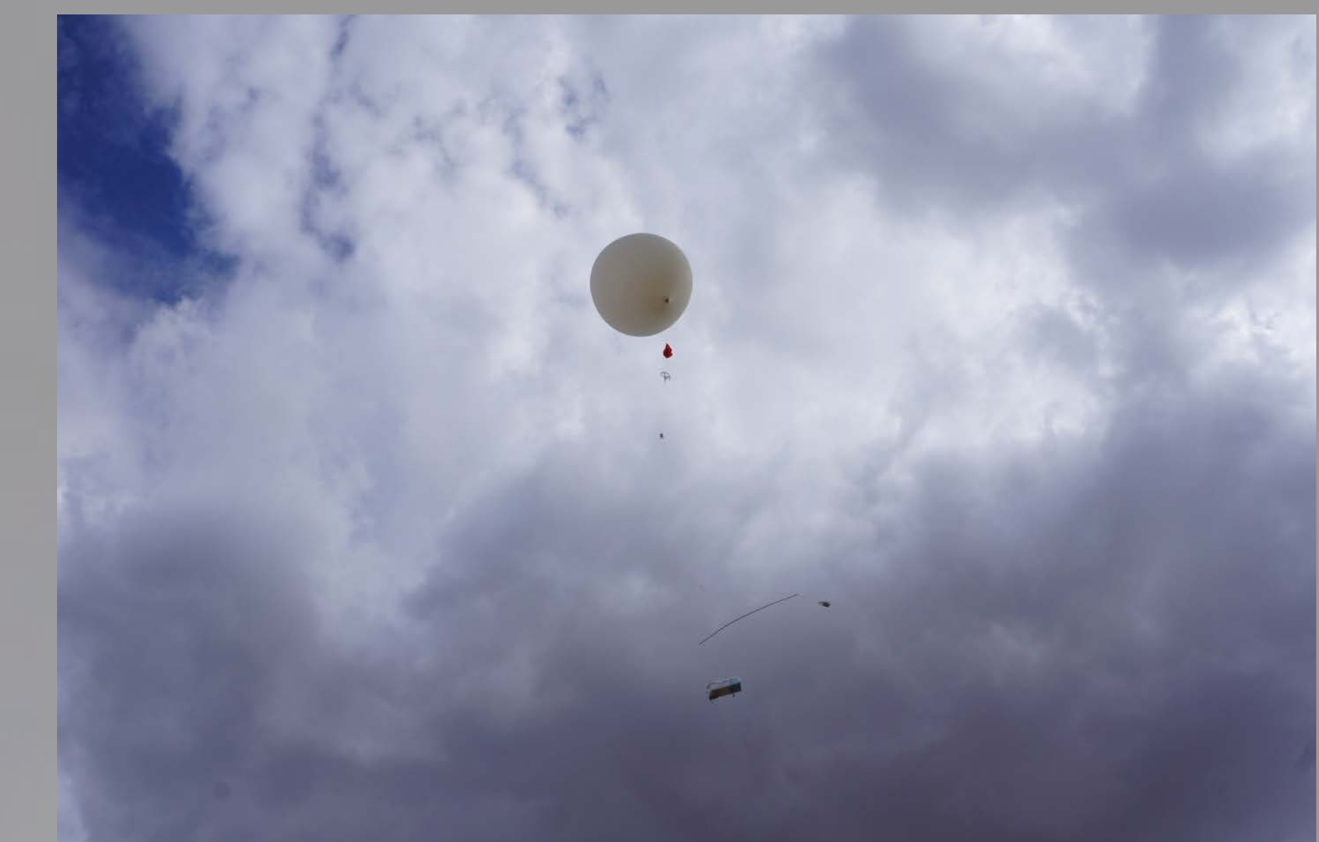
Launch package consisting of the CFH and the RS-92 radiosonde combination.
