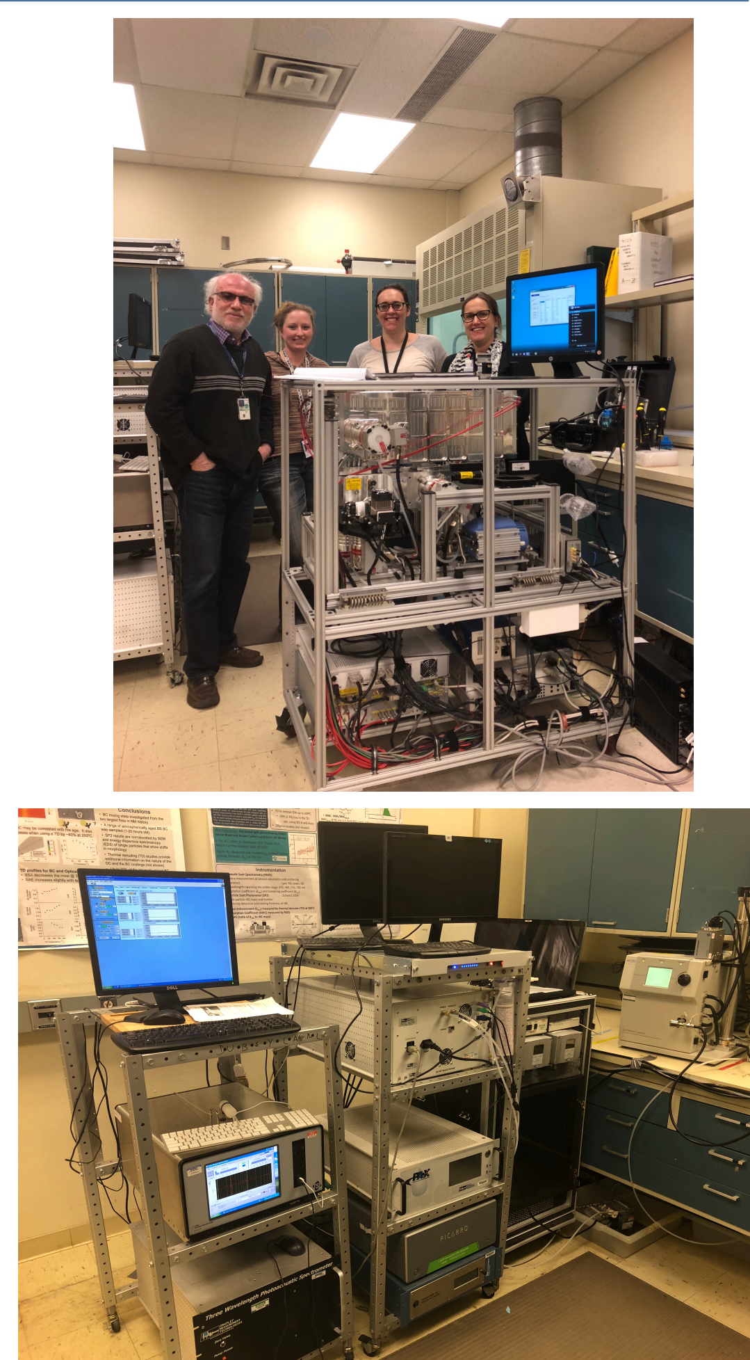
Fig 2. Humidified Nephelometer Calibrations, Repeatability and Optical and Chemical Instruments ➤ Humidity controlled dual nephelometer. ➤ Photoacoustic absorption & nephelometer. ➤ Size distributions with SMPS and laser sizer. ➤ Bulk off-line & SP-AMS chemical analysis.
