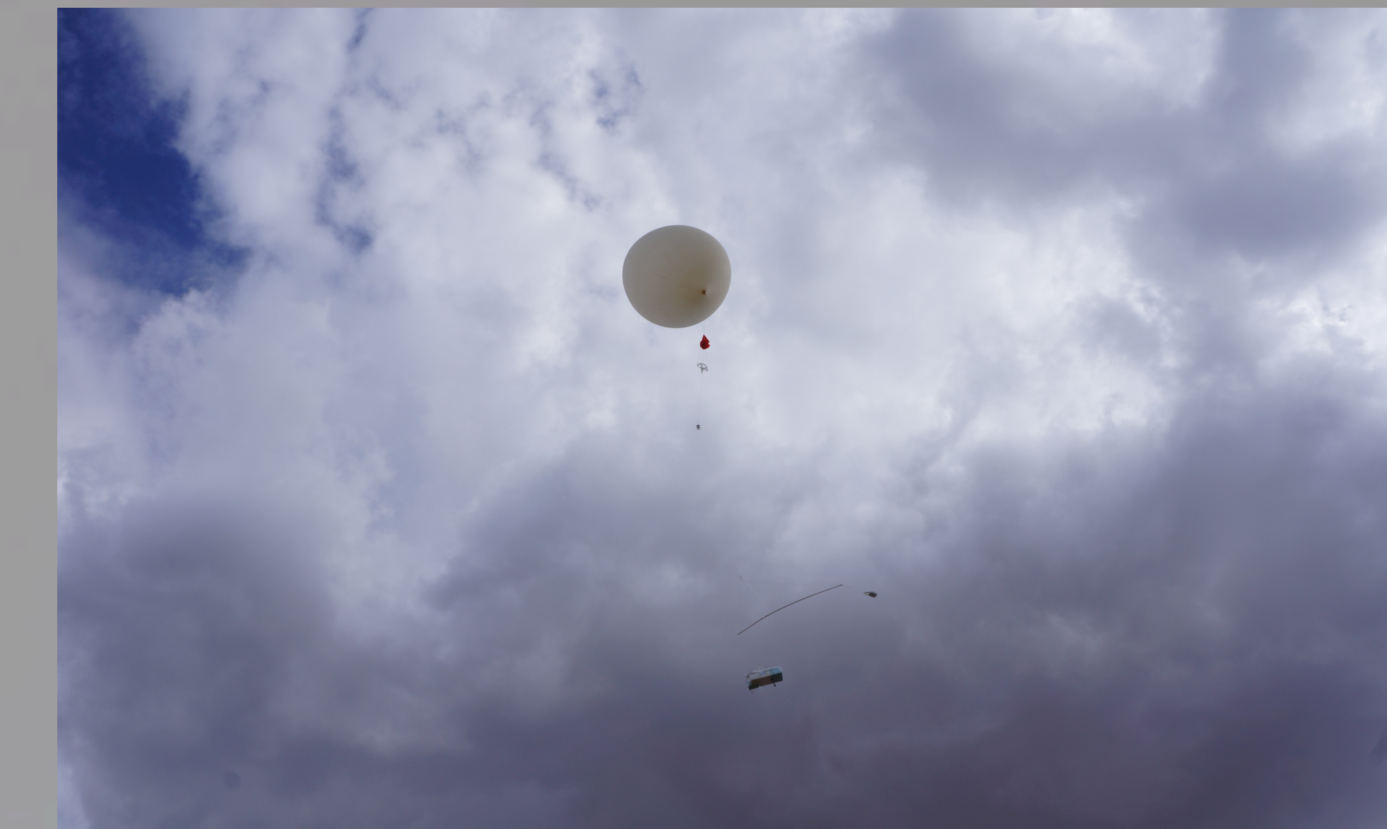
Launch package consisting of the CFH, iMet, and the RS-92 radiosonde combination.
