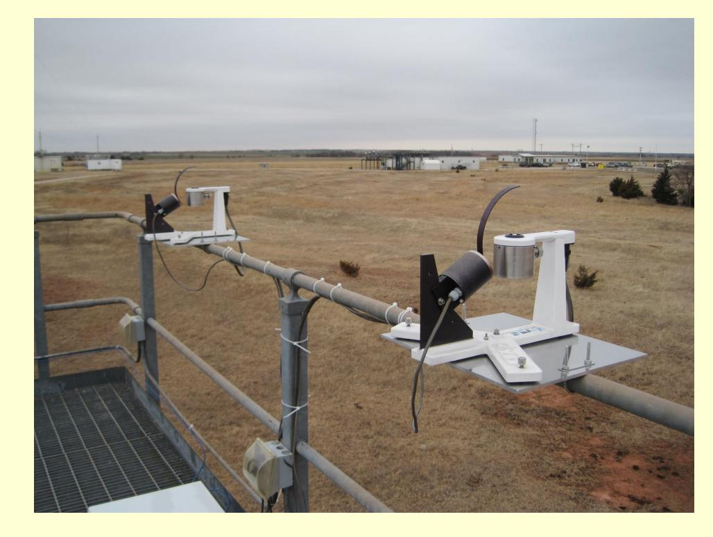
**Feb 2018:** Two new model MFRSRs installed on GIF. One will deploy with BRS instrument suite, and the other will be a spare. These instruments utilize a thermopile detector for broadband measurements, an improvement over the prior unfiltered silicon detector. The motor bracket has three fixed positions easing set-up and shadowband alignment. Head temp is maintained at 45°C so will stay above ambient thereby improving stability.
