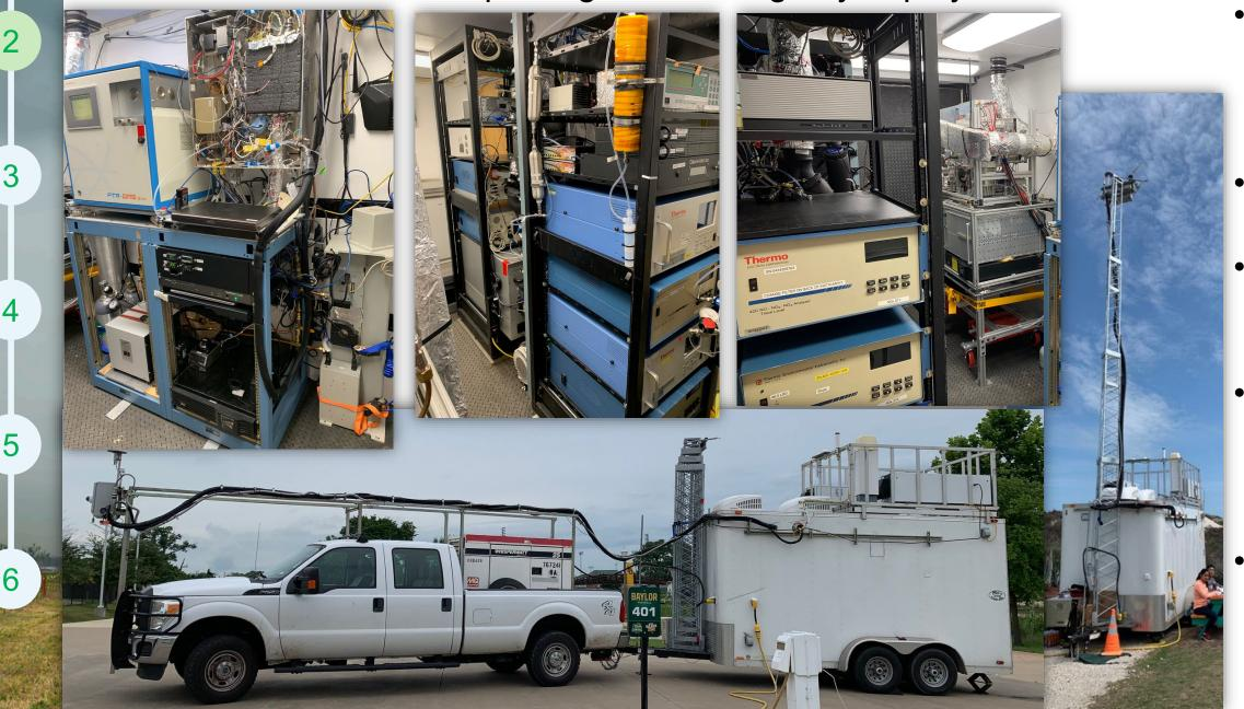
• A generator keeps instruments running during transport between sites. The sample tower extends 30 ft. • AC is plumbed directly to each instrument. Instruments can be checked remotely when stationary or in transit. Aerosol, trace gas and VOC have collocated inlet lines.
