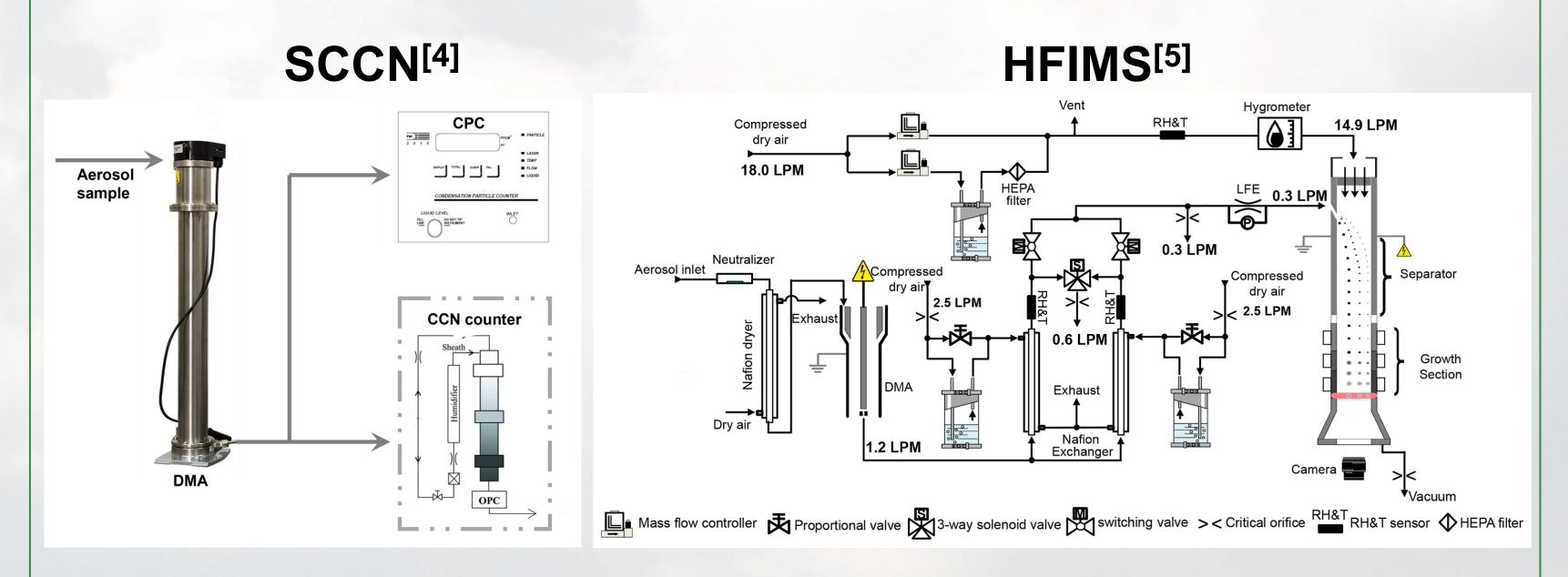
Supersaturation range: 0.08 – 1.8% Particle sizes: 40, 50, 75, 110, 165 nm Time resolution: ~1 hour
