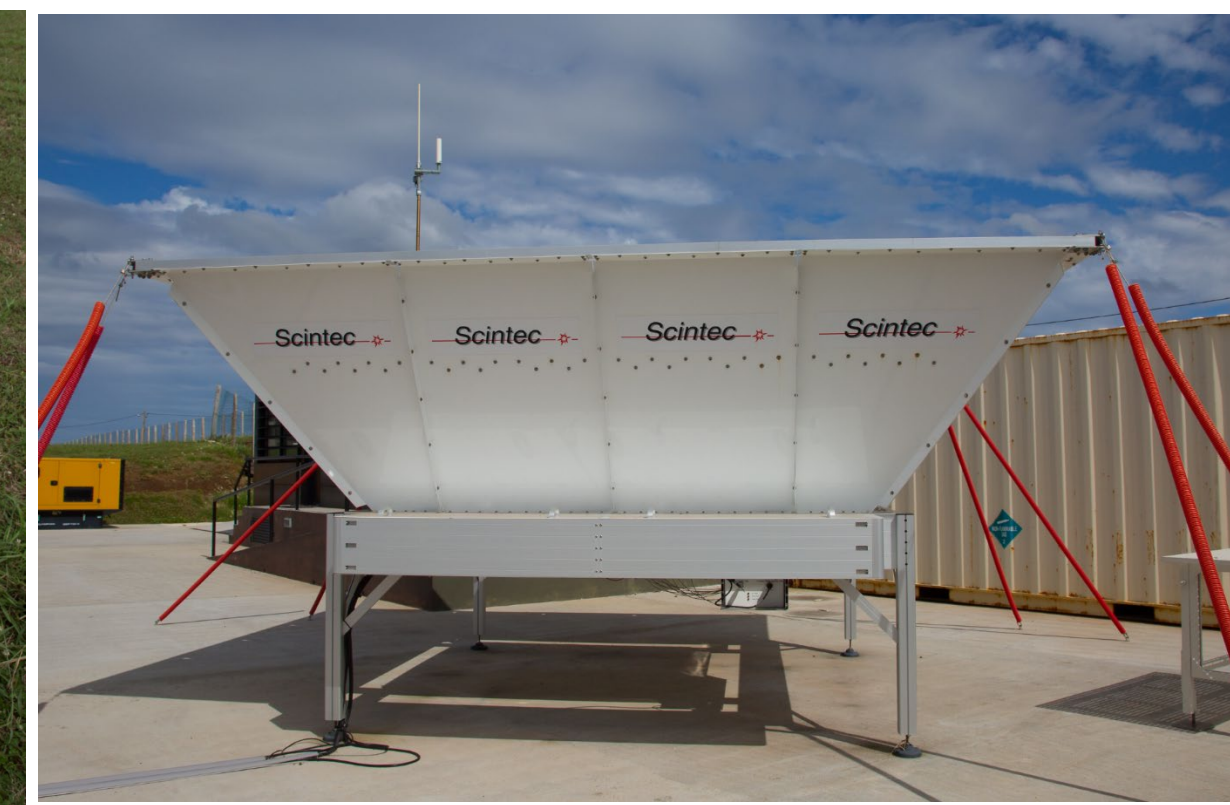
Radar Wind Profiler (RWP) at ENA
