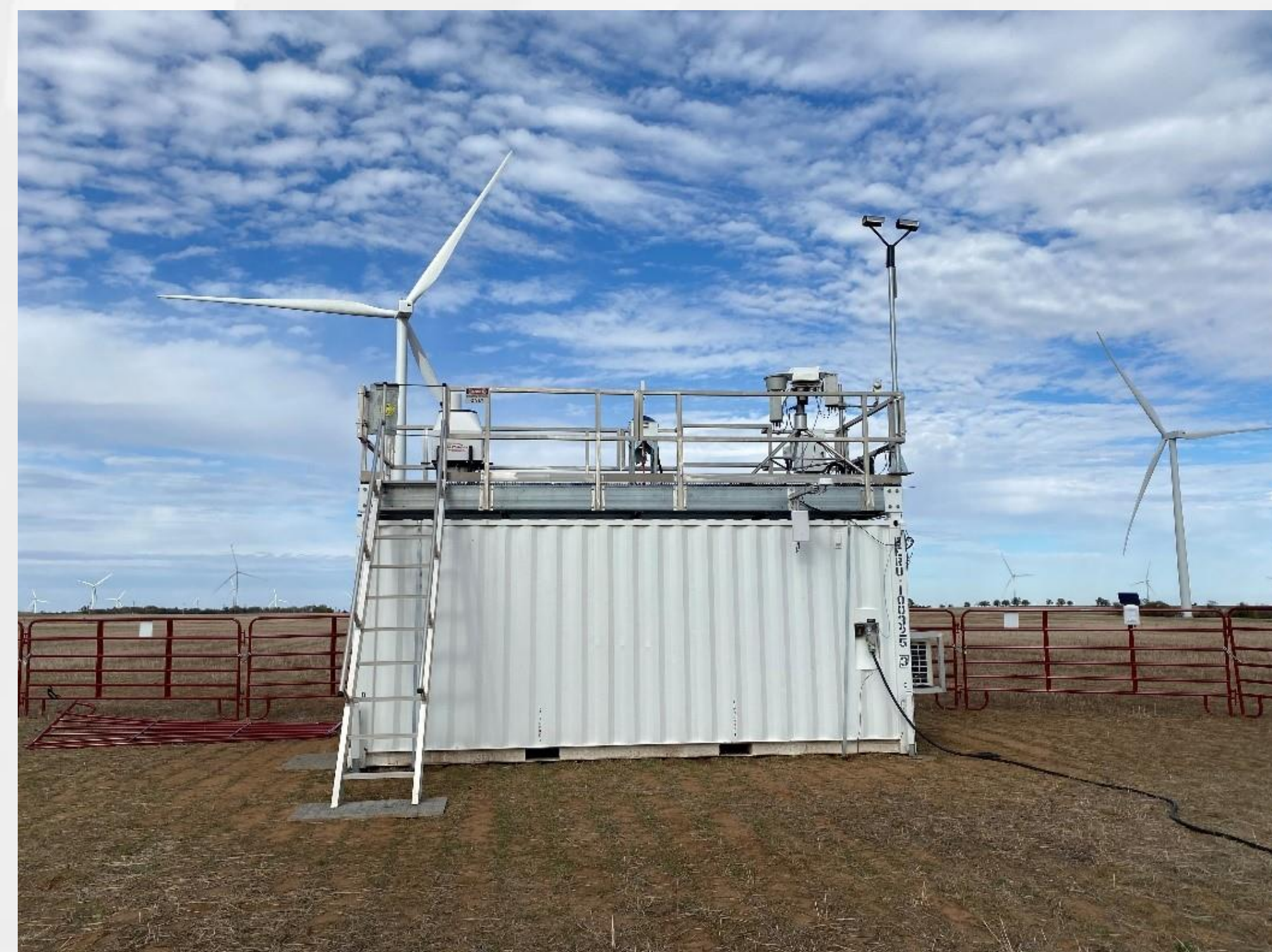
Figure 1: ARM AMF-3 instruments including a scanning lidar at AWAKEN site A1.
