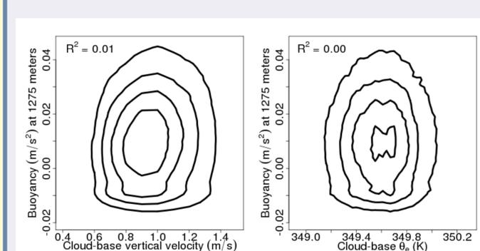
Figure 2: For cloudy parcels, a scatterplot of 1275-meter buoyancy versus cloud-base  $w$  (left) and cloud-base  $\theta_e$  (right).
