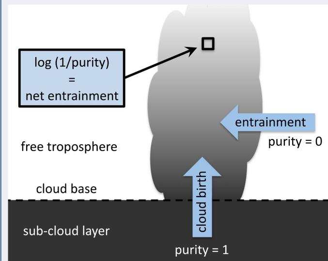
With an additional “theta-e tracer” – set to  $\theta_e$  below the cloud base and 0 above – we can encode the cloud-base value of  $\theta_e$  in the cloudy parcels. Since entrainment dilutes the two tracers by the same fraction, their ratios are unchanged. Therefore, the ratio of the two tracers is equal to the parcel's cloud-base  $\theta_e$ .
