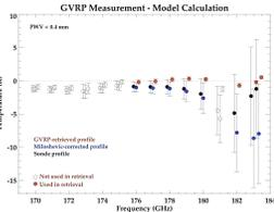
The retrieval produces WV profiles that result in residuals with small biases and standard deviations across all GVRP channels used in the retrieval.
