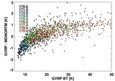
Model-measurement residuals (using scaled sonde profiles) indicated disagreement when the BT < -11K. No uncertainty in the model is large enough to explain this disagreement.
