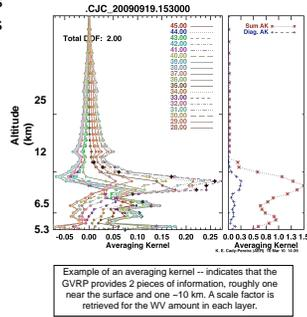
Example of an averaging kernel - indicates that the GVRP provides 2 pieces of information, roughly one near the surface and one ~10 km. A scale factor is retrieved for the WV amount in each layer.
