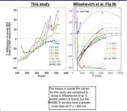
The biases in sonde RH values for this study are compared to those in Milosheovich et al. A similar pattern is found, but the RHUBC-II sondes have a greater moist bias for P > -400 mb.
