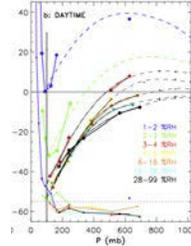
Daytime mean percentage bias of RS92 sondes relative to frost-point hygrometer measurements. This is the basis for the 'Milo' correction.
