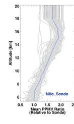
On average, the Milo correction leaves the near-surface water vapor unchanged and increases it higher up. The effect on PWV is a net increase of ~10%.
