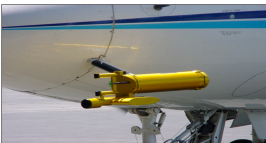
Figure 3. Photograph of the CAPS instrument fixed to the DOE G1 aircraft.
