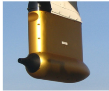
Figure 1: Photo of CPI installed on Convair-580 during ISDAC
