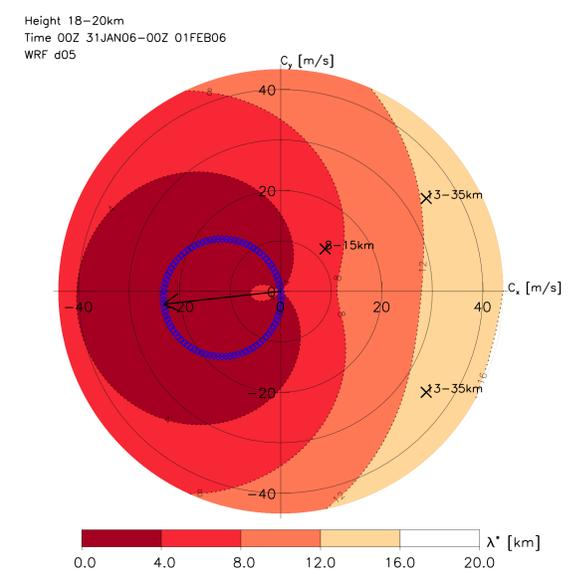
Figure 5: The critical wavelength  $\lambda^*$  as a function of phase speed from Run 2.  $c_x$  and  $c_y$  are the zonal and meridional phase speeds. The arrow represents the mean wind in the layer. The blue circle mark possible critical layers. The crosses mark the phase speeds from the model spectra (Fig. 4) and the corresponding range of horizontal wavelengths.
