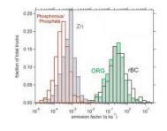
Emission factor distributions for major and minor chemical components of exhaust particulate matter from diesel trucks.
