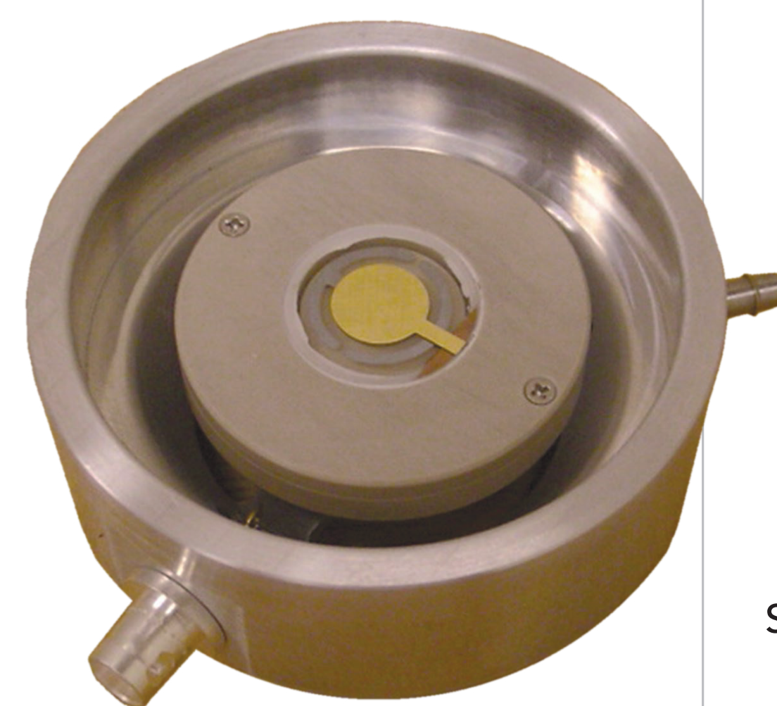
Figure 3—QCM mounted to an impaction plate
