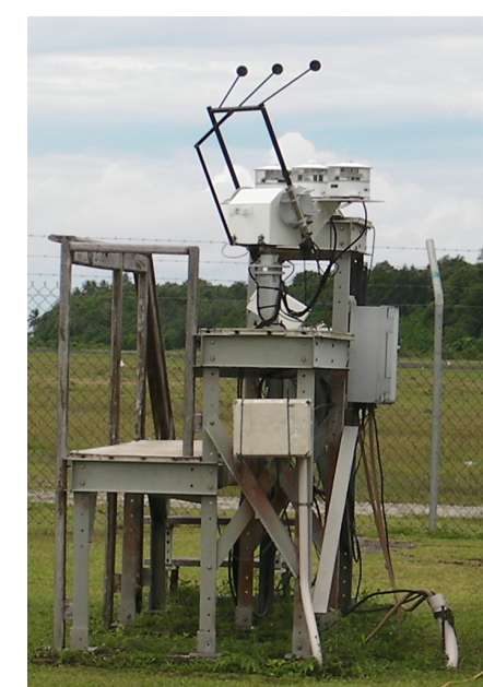
Radiometers at standard Manus site
