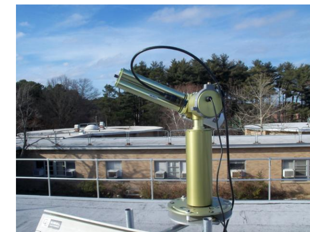
L. Gregory: CSPHOT on top of Bldg. 490 at BNL doing a direct Sun observation during the 2011 Aerosol Life Cycle Field Campaign.
