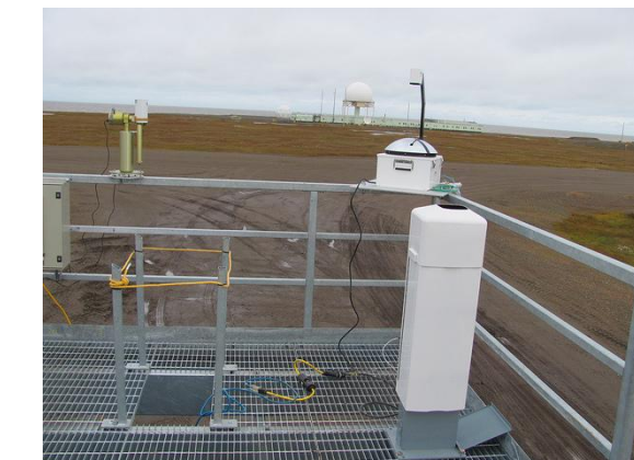
AMF3 site ops: CSPHOT installed at Oliktok, Alaska
