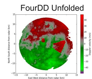
Raw and unfolded velocities from the ARM CSAPR radar in the SGP corrected using FourDD [1]. Data is from the first 150 gates of a PPI scan at the highest elevation (42°) collected at 10:47 UCT on May 20, 2011
