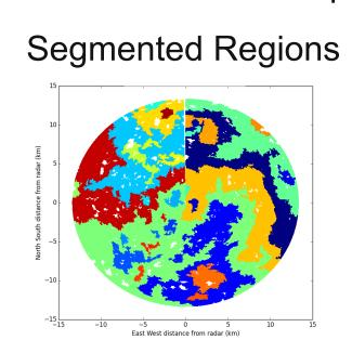
These regions are then unwrapped against each other by minimizing the velocity differences between all bordering gates. Regions with the largest number of shared edges are unwrapped fist. This step is accomplished by modeling the regions and edges as a dynamic network graph.
