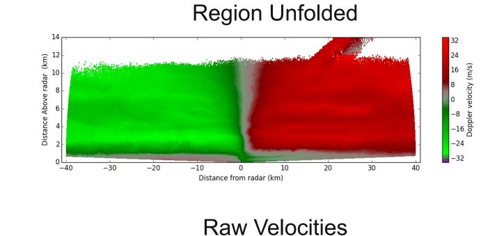
Doppler velocities from the ARM XSAPR at the SGP I5 site collected at 11:36 UTC on May 20, 2011. Data is from an RHI scan. Gates with reflectivity below -5 dbZ were excluded when unfolding.
