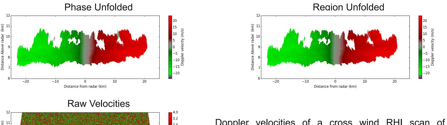
Doppler velocities of a cross wind RHI scan of the WSACR instrument in the SGP collected at 20:40 UTC on August, 20, 2012. A feature mask from the currently indevelopment SACRCOR VAP was used to select gates and suppress returns from noise, clutter and insects.
