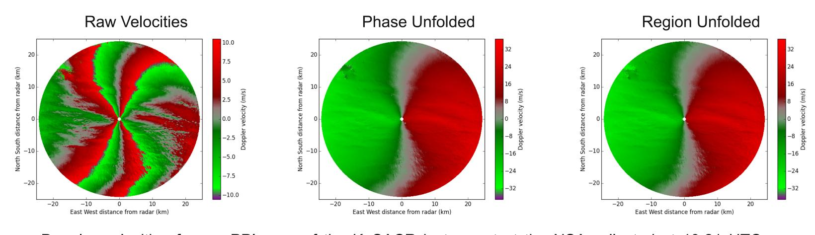
Doppler velocities from a PPI scan of the KaSACR instrument at the NSA collected at 13:21 UTC on January 14, 2014. Data is from the 1° elevation scan, no gates were excluded when unfolding.
