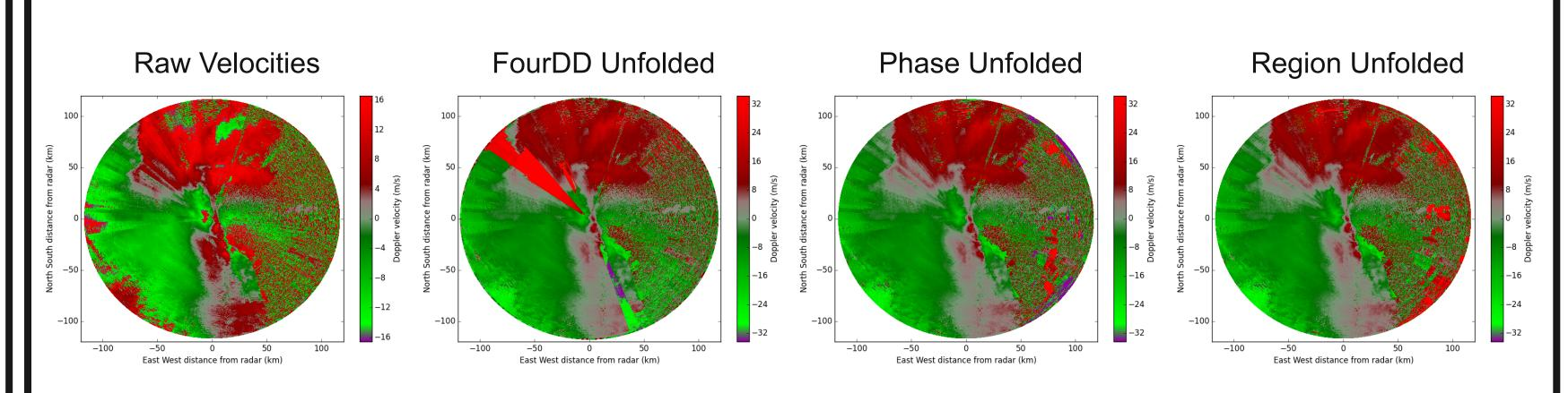
Doppler velocities from the ARM CSAPR radar at the SGP site corrected using FourDD [1], multi-dimensional phase unwrapping, and the region based dealiasing algorithms. Data is from the lowest PPI scan with an elevation of 0.75° collected at 10:47 UTC on May 20, 2011.
