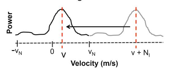
Various algorithms have been designed to unfold or dealias the measured velocities to determine the true atmospheric velocities. Unfortunately when applied to data from ARM's scanning radars, these algorithms often produce imperfect results.
