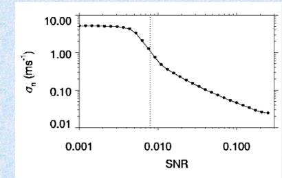
Figure 2. Radial velocity precision as a function of SNR. The radial velocity precision is used to estimate measurement uncertainty for trial 3.
