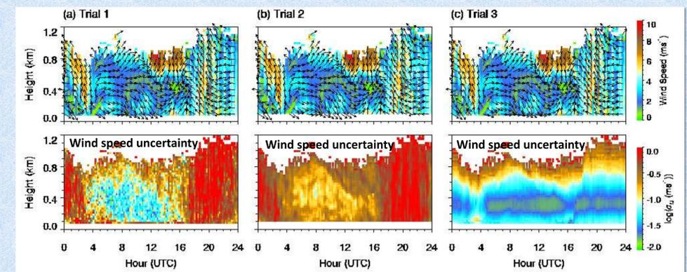
Figure 3. Time-height cross sections for 9 March 2015 showing retrieved winds (top) and estimated wind speed uncertainties (bottom) for a) Trial 1, b) Trial 2, and c) Trial 3.
