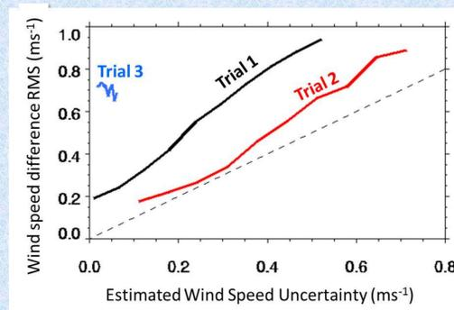
Figure 4. Root-mean-squared difference in wind speed between the lidar and tower wind speed as a function of the estimated lidar wind speed uncertainty. The black, red and blue curves show the results for Trials 1, 2 and 3 respectively.
