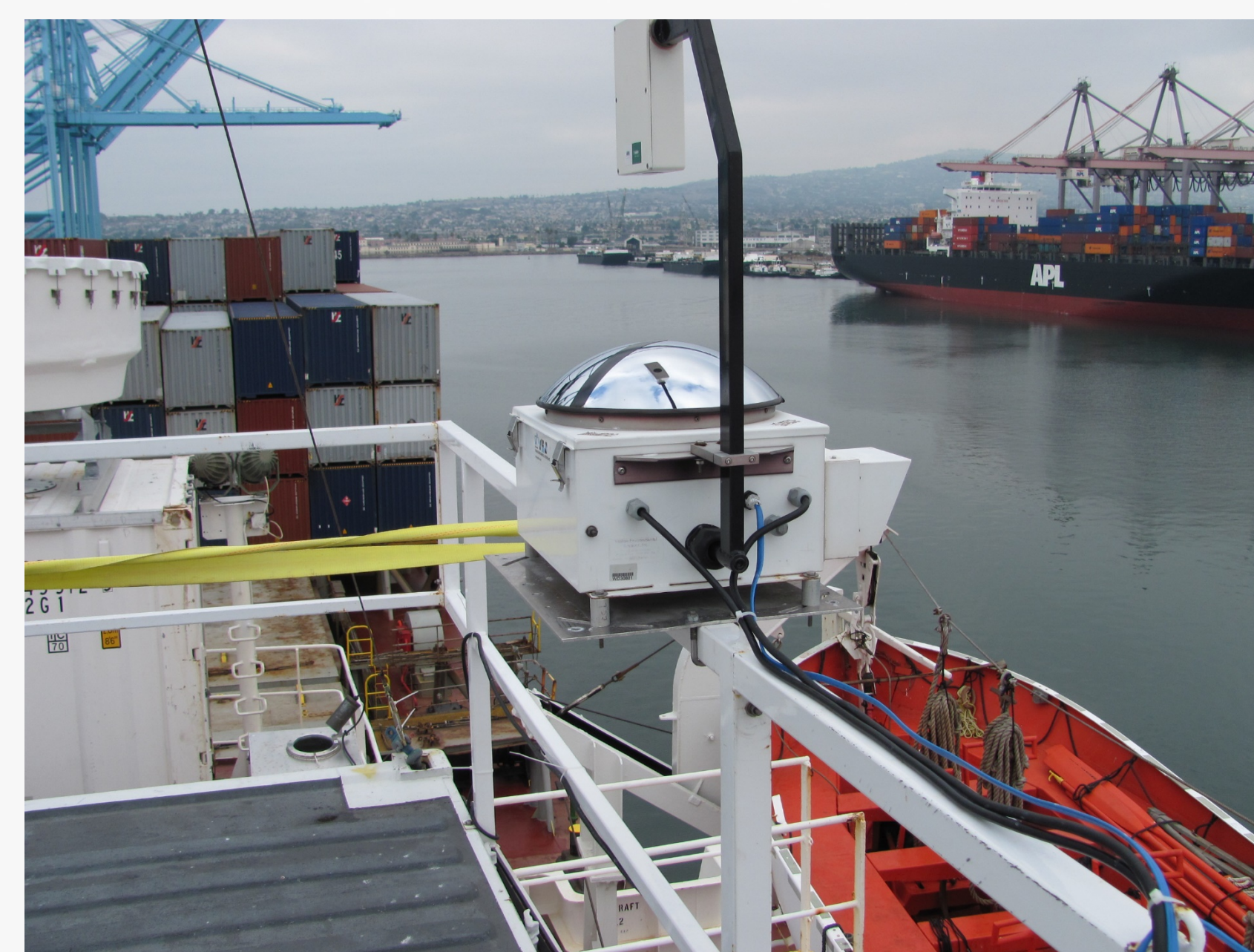
Total Sky Imager installed on the Horizon Lines Spirit for MAGIC.
