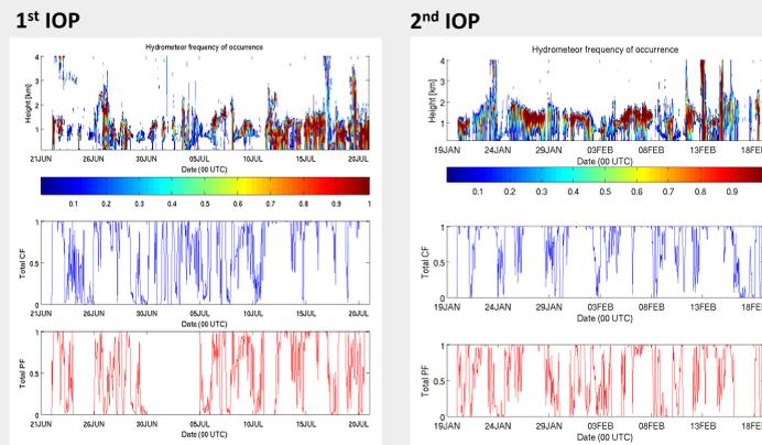
(top) Hydrometeor frequency of occurrence from combined cloud radar, micropulse lidar and ceilometer observations (Kollias et al. 2007). (middle) Total cloud fraction. (bottom) Total precipitation fraction (precipitation defined as radar echo below ceilometer cloud base height).
