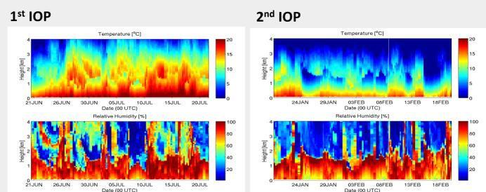
(top) Time series of the profile of dry bulb temperature from radiosonde observations (bottom) same for relative humidity.
