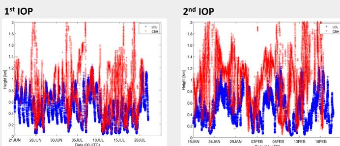
Time series of lifting condensation level (LCL) from surface meteorology measurements and the lowest cloud base height (CBH) as observed from the ceilometer.
