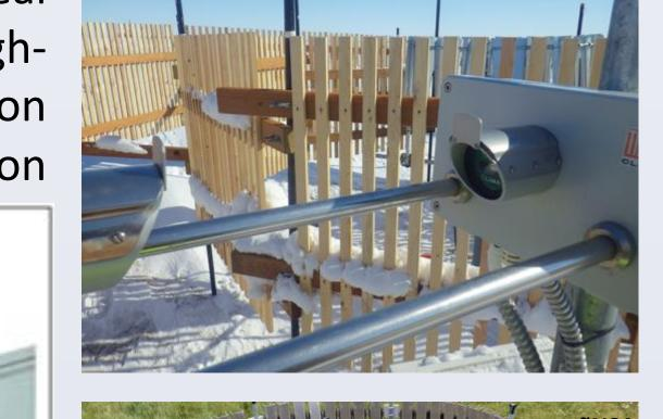
An outside laboratory is also being established at University of Alaska Fairbanks to monitor the performance of the newest instrumentation (LPM, WBGEONOR, SRS) under adverse conditions to come up with guidelines for operation at NSA and OLI.
