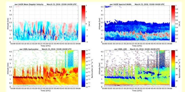
Figure 1. Example of radar data from AMF-2 at Ross Island showing extremes in vertical velocities that are an order of magnitude larger than normally observed in Arctic clouds. Also structural complexity in mixed-phase clouds seen in High Spectral Resolution Lidar (HSRL) data.
