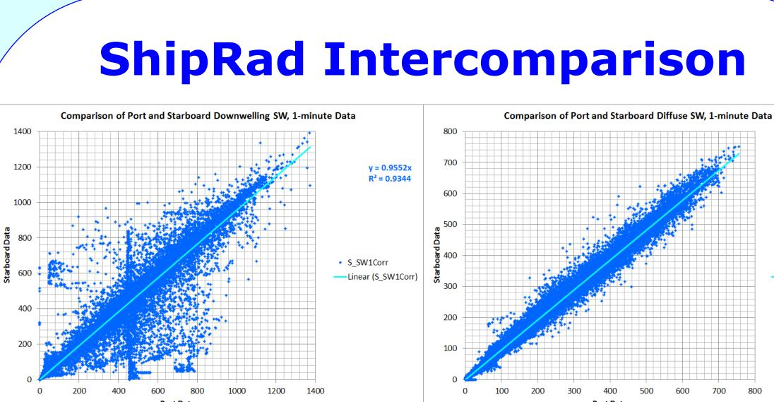
Large disagreements between port and starboard downwelling SW (left plot) are due to shading of one of the systems. The diffuse SW (right plot) does not show similar disagreements because the diffuse is already a shaded measurement.
