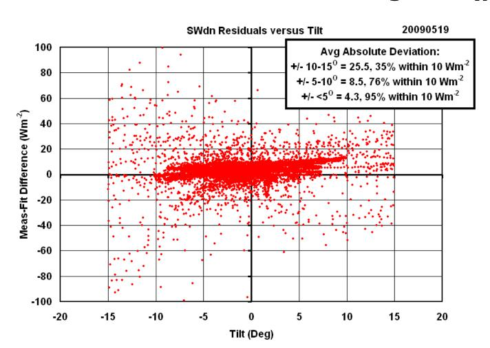
Long et al. (2010) show that the tilt correction methodology corrected 90% of the data to within 10 Wm<sup>-2</sup> for tilt of  $+/-10^{\circ}$  or less, with an average absolute deviation of  $5.2 \text{ Wm}^{-2}$ , and 95% if the data within 10 Wm<sup>-2</sup> for tilt of  $\pm/-5^{\circ}$  or less.
