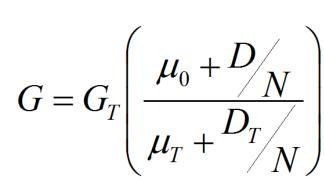
from tilted SW ( $G_{\tau}$ ). N is direct normal SW, D is diffuse SW (assumed to be equal for modest tilt),  $\mu_0$  is the solar zenith angle, and  $\mu_T$  is the tilt zenith angle = f(pitch, roll, heading)
