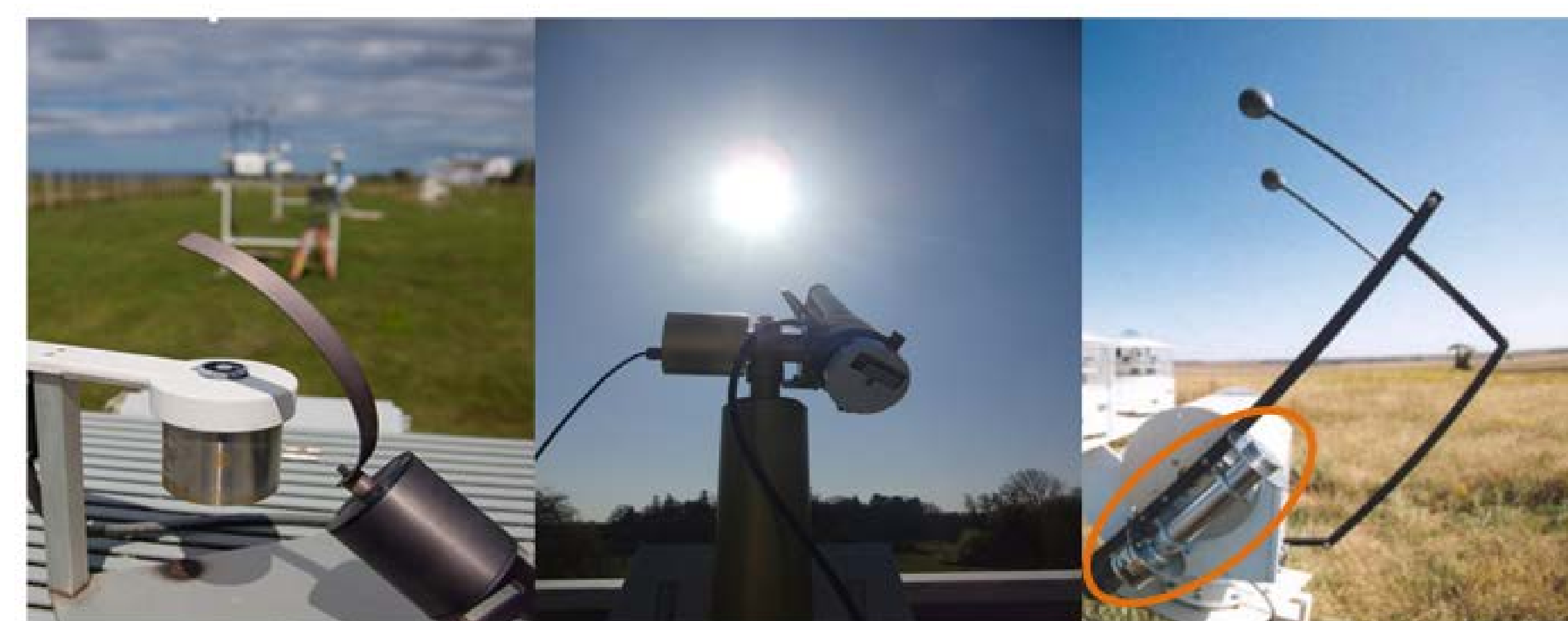
Images of three ground-based instruments for measuring AOD: MFRSR (left), CSPHOT (center) and NIMFR (right)
