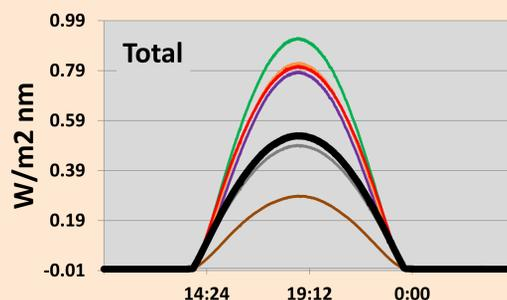
The first deployed sensor with a 1625 nm filter detector in place of the unfiltered silicon detector is at SGP EF-38. Provided is a set of typical MFRSR plots showing direct, diffuse, and total irradiance. Note the calibration value for 1625 nm is yet to be determined, so plots are for illustration purposes only.
